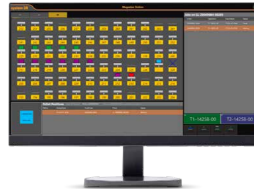
Magazine manager– Function for direct job control (independent loading, job assignment, etc.)
